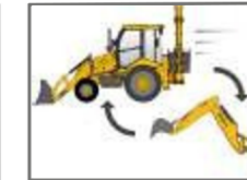
Effy power selector switch Wheel drive / backhoe
